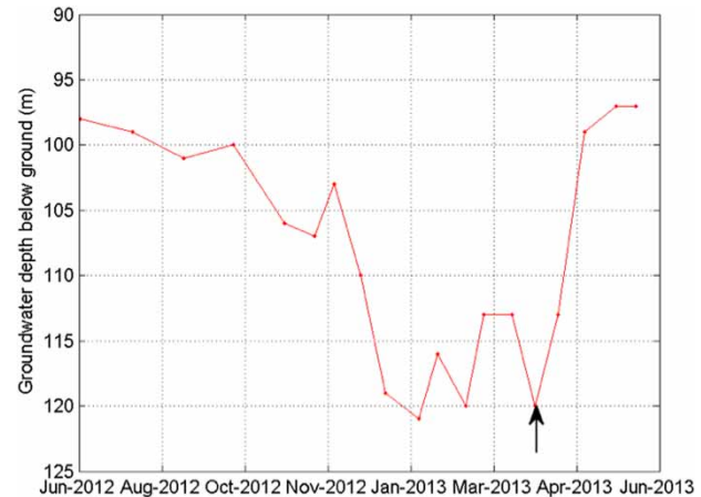
Figure 4 | Borehole water levels at a site within the study area, Mogwadi (Dendron) (arrow indicates application of pumping restrictions).
